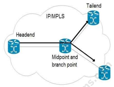
An engineer is implementing an MPLS P2MP TE solution. Which type of router can serve as the midpoint router and the tailend router in this P2MP TE network implementation?
